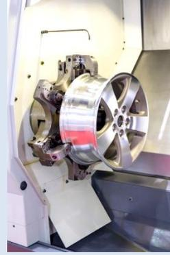
A variety of alloy rims with different dimensions (17"–22" inch diameter) had to be accommodated at a production rate of 300 rims / hour.
